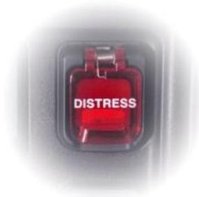
The simplest component/feature of a VHF-DSC radio is the DISTRESS button. Simply pressing it, transmits an immediate distress call to other ships in range and the USCG along with your ship's ID and location. Then, follow-up broadcast notification and communication can transpire on VHF Ch 16 as shown below.
